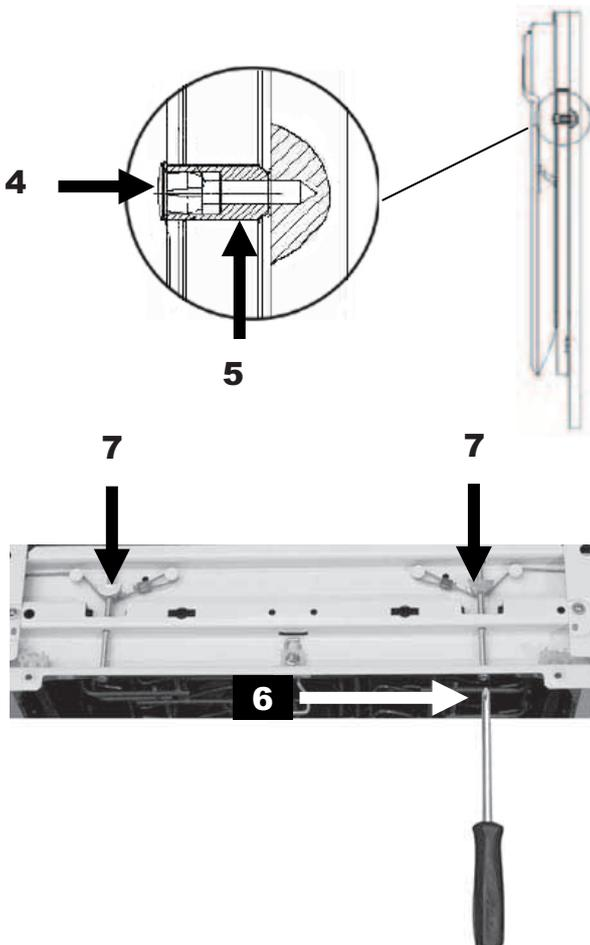
The door springs are set at the factory to the proper tension for the outer door. If aesthetic wooden panels are installed, you will have to adjust the door spring tension. Rotate the adjusting screw **6** to drive the adjuster **7** to strain or relax the steel cable.
