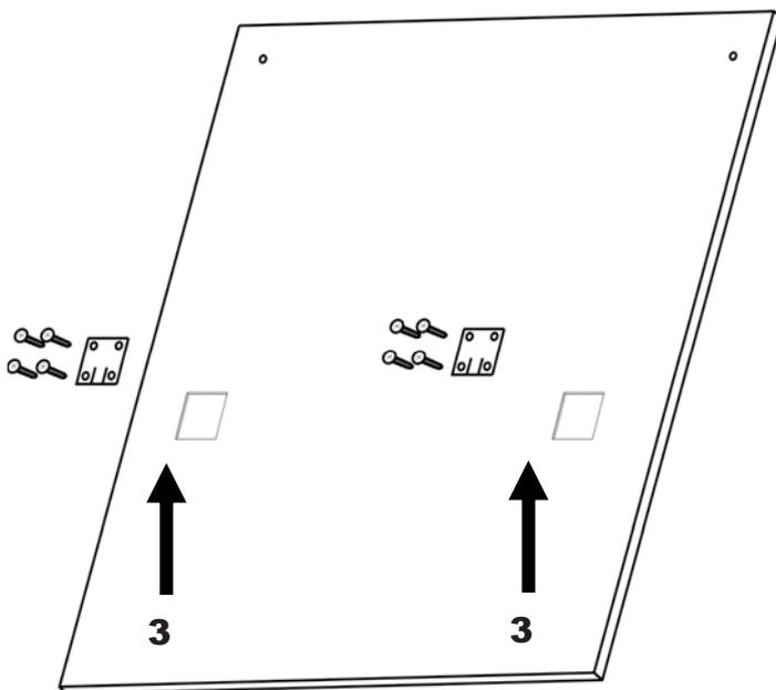
Install the bottom hooks from the interior of the furniture door by countersunk head screws **3**.
