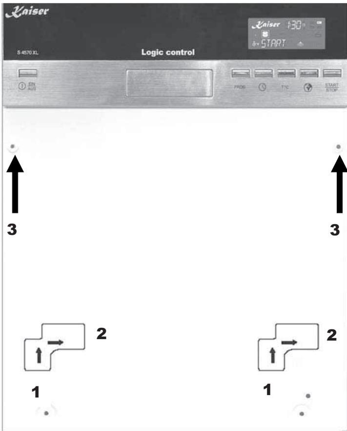
The hook is lifted from position **1** to the appropriate place, and then pushed right to the position **2**, making the panel and the outer door align.
