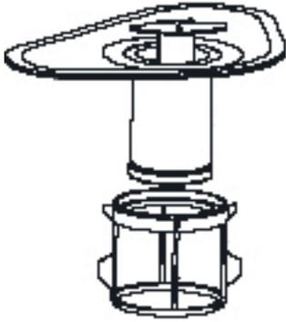
To clean the coarse filter and the fine filter, use a cleaning brush.
