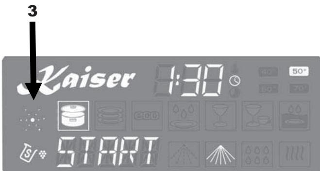
The rinse aid should be added, when the Rinse aid warning light **3** on the information display goes on.
