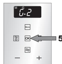
The display **2** shows a symbol **3**, **G** to display a kind of operating function and a symbol **4**, **G.** to display it's variant.
