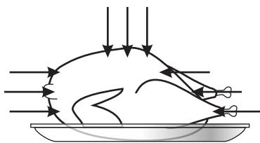
The friction between molecules produces heat which raises the temperature of the food, de-freezing it, cooking it or keeping it hot.
