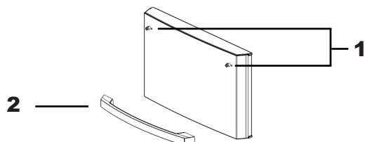
Use cross recessed screwdriver to set the bolts **1** on the door as shown in the figure. Fix them tight on the door. Place the handle **2** from above as per the direction shown at the picture and hang the handle above on the set bolts. Using the supplied hexagon spanner set screws into the threaded holes and tighten them gently. Ensure that the handle is well erected.
