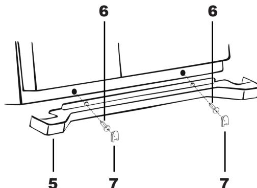
Install the decorative bar **5** on the bottom panel as shown in the figure. By means of a cross recessed screwdriver turn the screws **6** to tighten. By means of delivered in the complete set screw caps **7** close openings for screws. Remove a protective film from the bar.
