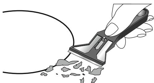
First of all remove stray food bits and grease drops from the cooking surface with the special scraper. Then clean the hot area as best as possible using non-aggressive detergent then rinse again with water and dry with a clean cloth.
