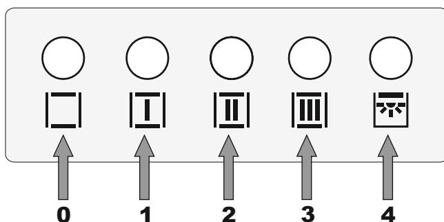
The button **4** is used to turn on and off the extraction hood lighting; independently of the engine work status, push this button to switch on/ off the lighting. Its indicating light turns on/ off accordingly.
