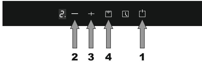
After connecting the cooker hood to the main supply, the back light of the keys is turning on. The back light will turn off after 30 seconds without any operation and the cooker hood will enter into stand-by mode.
