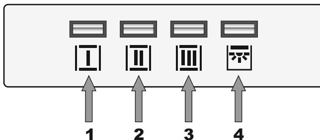
**Upper picture.** The buttons **1**, **2** and **3** serve the purpose of selection of the engine speed in range from 1 to 3.
