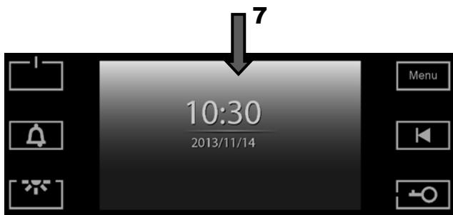
1. ON/ OFF key – to switch the appliance on and off
