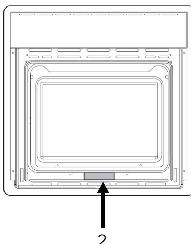
**Attention!** After converting the appliance to a different type of gas, remember to change the data plate 2 to one with the new data (gas type and pressure)
