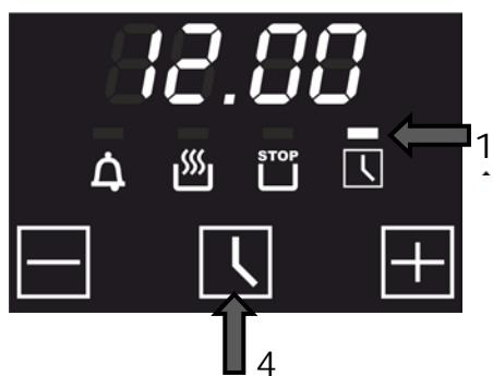
After a few seconds the controller sets the time currently displayed and the symbol 1 goes out.
