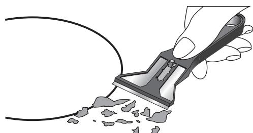
Pieces of aluminum foil and plastic material which have inadvertently melted or sugar remains or highly sacchariferous food have to be removed immediately from the hot cooking area with the special scraper. -This is to avoid any possible damage to the surface of the top.
