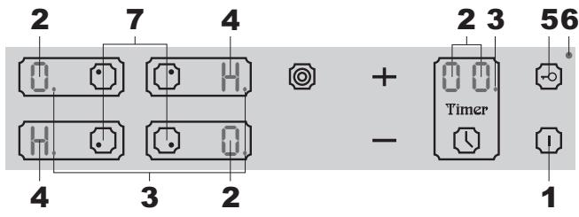
It comes a sound signal. The displays of the heating fields and of the timer show the symbols **2 (0)**, the symbols . (dots) **3** blink. If a cooking zone has residual heat, the display shows a symbol **H, 4**.
