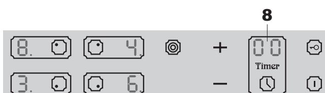
When the set time has elapsed, an acoustic signal is emitted, the heating zone turns off. On the timer display **8** blinks **00**.
