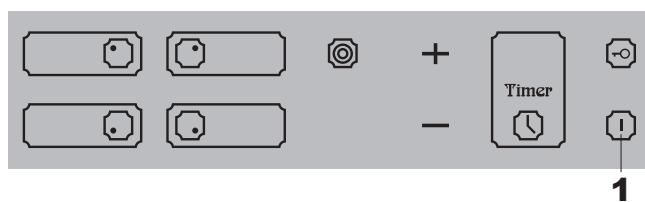
Be especially careful to keep the sensor keys clean since soiling could be mistaken for finger contact by the appliance. Never put anything (pans, tea towels etc.) onto the sensor keys! If food boils over onto the sensor keys, we advise you to activate the **OFF** key **1**.
