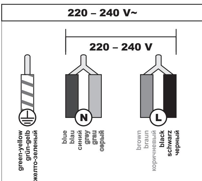
If the appliance is to be connected directly to mains terminals, fit a switch with minimum aperture of 3 mm between the contacts. Make sure that the switch is of sufficient capacity for the power specified on the appliance's data plate, and compliant with applicable regulations. The switch must not break the green-yellow earth wire. The socket or switch must be easily reachable with the cooking hob fully installed.
