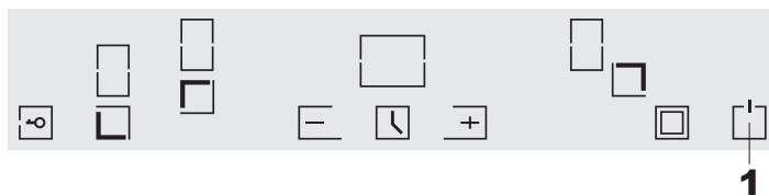
Be especially careful to keep the sensor keys clean since soiling could be mistaken for finger contact by the appliance. Never put anything (pans, tea towels etc.) onto the sensor keys! If food boils over onto the sensor keys, we advise you to activate the **OFF** key **1**.
