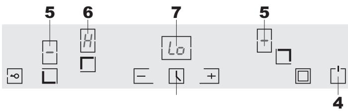
After mains voltage is applied the control initializes for approx. 1 second before it is ready for operation.
