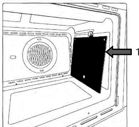
Our smooth walled ovens can be fitted with self-cleaning panels 1 to cover the inside walls.
