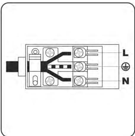
If the appliance is to be connected directly to mains terminals, fit a switch with minimum aperture of 3 mm between the contacts. Make sure that the switch is of sufficient capacity for the power specified on the appliance's data plate, and compliant with applicable regulations. The switch must not break the yellow-green earth wire. The socket or switch must be easily reachable with the oven fully installed.
