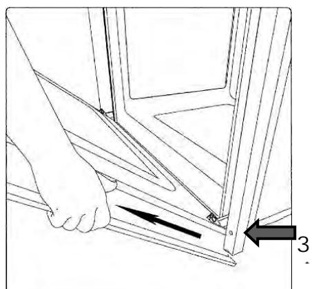
The track system is easily to be removed to clean the oven. The construction is made of stainless steel, which excludes the possibility of corrosion formation.
