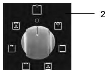
Oven operation functions are steered through turning of the rotary knob temperature regulator 1 and rotary knob mode of operation 2 on the control panel 3.
