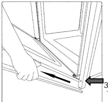
The tracks of every griddle resist a loading up to 15 kg in the completely pulled out state.
